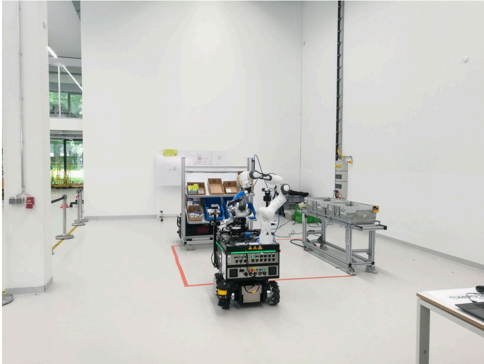
Figure 4: Demo area for the milestone 2 demonstration at the stakeholder meeting in June 2023. In front of the robot is the shelf with objects to be picked, and to the right is the table with trays where objects should be placed.
